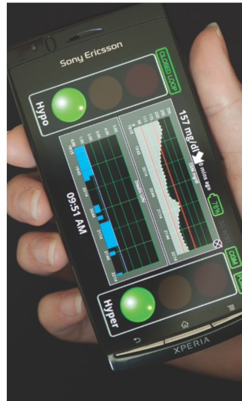
Closed-loop algorithms can run on smartphones; this version shows insulin delivery and glucose level.
