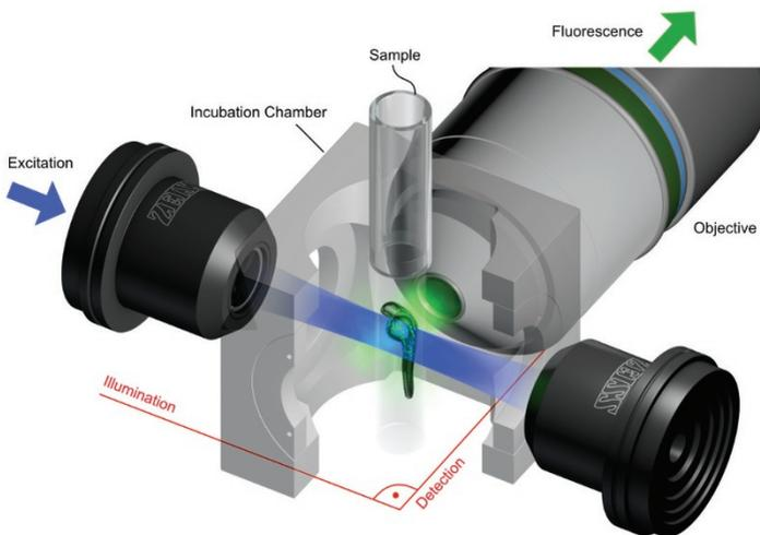
**Figure 1.** In LSFM, fluorescence excitation (blue arrow) and detection (green arrow) are split into two distinct optical paths. The illumination axis is orthogonal to the detection axis. The LSFM concept is compatible with imaging in dedicated incubation chambers that keep the specimen in a close-to-natural environment over long periods of time. Reproduced with permission from ZEISS
