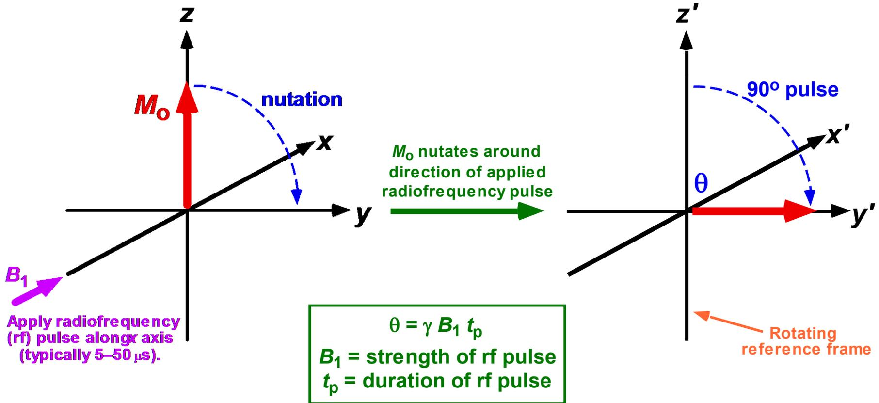
**A 90° pulse along the  $x$  axis will nutate the magnetization onto the  $y$  axis.**
