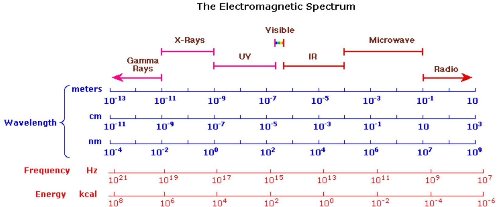
NMR uses electromagnetic radiation in the radio frequency range
