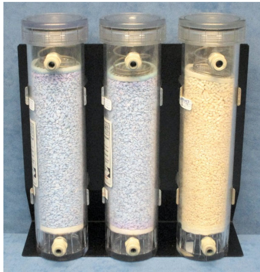
Two columns of Drierite and one column of Soda Lime
